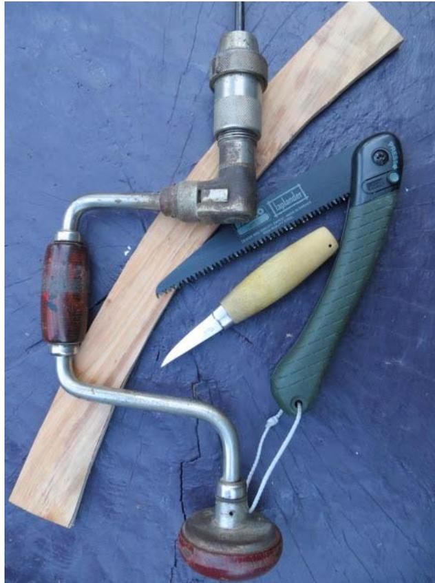
Tools for this project are simple: folding saw, small carving knife, drill and a wooden pattern.
