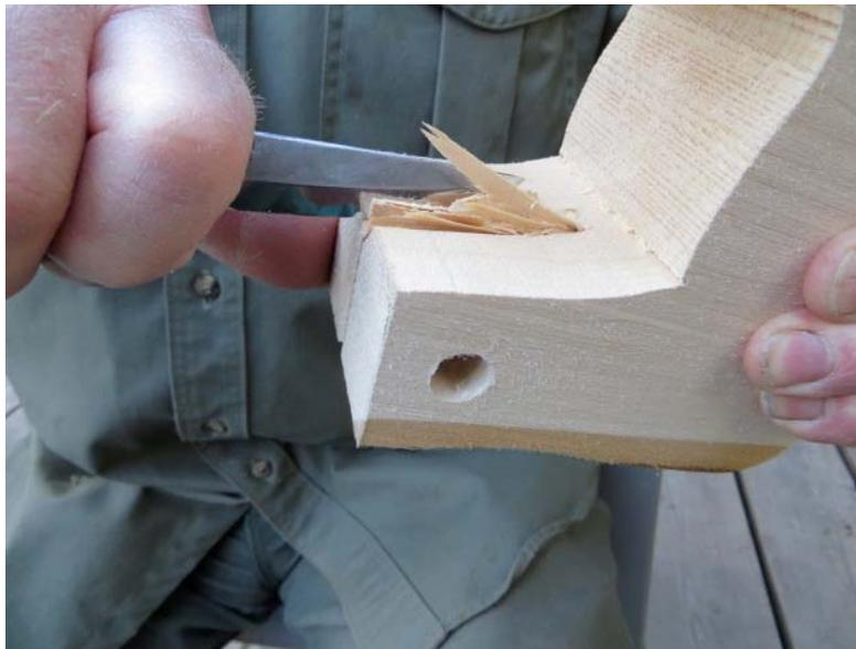
Use the belly of the blade to break away large chips between the legs. Do not be concerned with neatness, as neatness will take care of itself as you refine the shapes.
