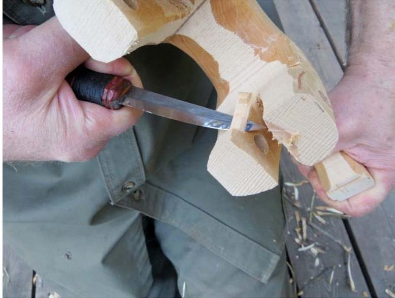
Using a chest lever grip is quite safe and will quickly remove wood from the hard-to-reach area between the legs.
